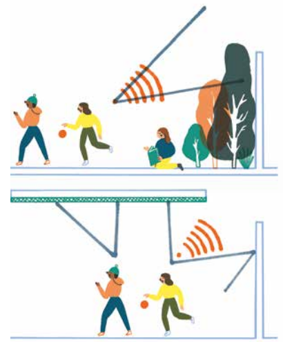
COMBINED SYSTEMS A wall that acts as a barrier to spreading noise and an absorbent roof or a greenery wall that increases its sound absorption coefficient by making it less smooth.
