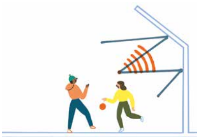
CONTAINING NOISE The wall prevents the spread of noise outside, but may increase noise inside the playground due to echoing.
